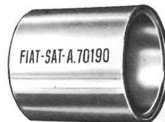
A.70190 Tool for fitting differential bearing inner race
