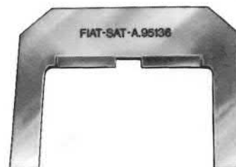
A.95136 Gage for checking float level
