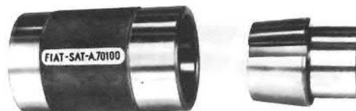
A.70100 Tool for installing circlip in 5th gear synchromesh unit
