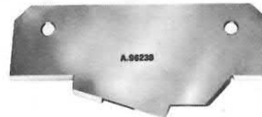
A.96238 Combustion chamber depth gage
