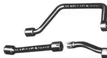
A.50131 Adapters for tightening 19 mm hex cylinder head nuts, intake side
