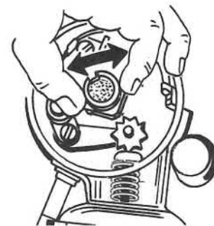
CHECK SIDE PLAY OF DISTRIBUTOR SHAFT
