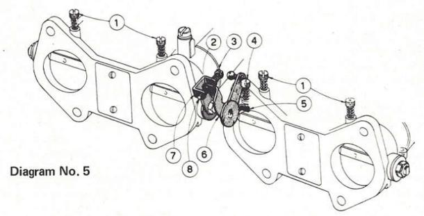
To ensure proper engine idle operation with paired WEBER DCOE series carburettors proceed as directed below.
