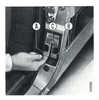
**Front Trunk** - To release, pull handle located underdash, lefthand side of steering post.
