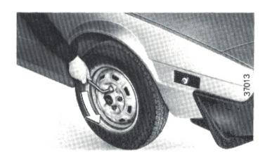
Using the wheel wrench slacken about one turn the mounting bolts.
