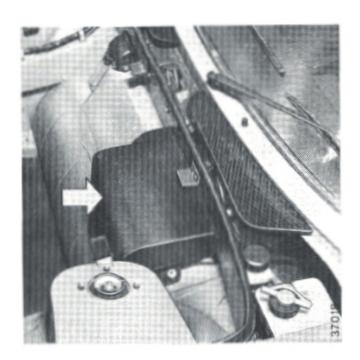
In hot climates check the electrolyte level more frequently than recommended.
