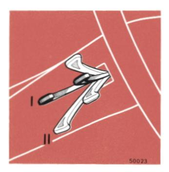
High/Low Beams Change-Over Switch Lever (With lighting switch pressed at Right)
