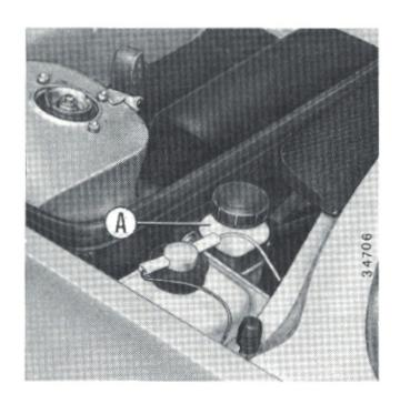
Clutch fluid topping up is an operation included in the Free Service Coupon.
