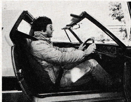
Door stays are weak on X1/9. Targa roof requires two people to lift it off and fit it into front boot. Seats are comfortable but lack rearward adjustment.
