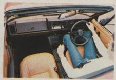
The dash now incorporates a lockable glovebox, regrouped instrument cluster and a new quartz digital clock. Switch gear is all new and is set into a moreattractive centre console, while there's also an upgraded sports steering wheel.
