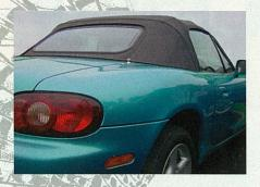
BAS are the only company in the world to produce a replacement hood, with a heated rear glass window, to the original specification of the Mazda MX5 Mk II.
